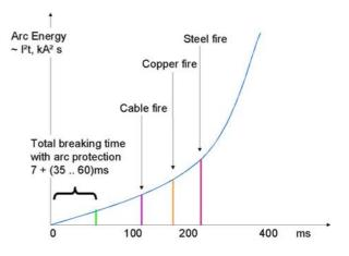
FIGURE 2: Arc energy as function of burning time. Points where metal parts start to burn are indicated. Arc protection will function before cable fire starts.
