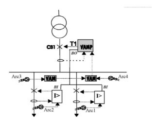
FIGURE 6: Overcurrent relays with arc sensor option and specialised arc protection system (VAMP and VAM). Information about activation of arc sensors Arc3 and Arc4 is also brought to the overcurrent relays via the binary inputs (BI).
