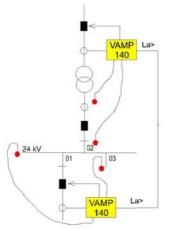
FIGURE 7: Arc protection system using overcurrent relays with arc sensor option. Information about the activation of the arc sensors may be carried between the relays using the binary inputs and outputs (La>).
